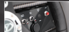
DASH PANEL W/STAINLESS TOGGLE SWITCHING, 12V & USB PORTS
